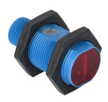
Contrinex photoelectric sensor, tubular, threaded, polarized retroreflective, visible red light emission, 0.02-7m sensing distance, complementary light-on/dark-on, NPN, 4-wire, 4-pin M12 quick-disconnect.
