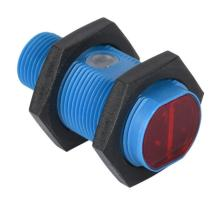
Contrinex photoelectric sensor, tubular, threaded, polarized retroreflective, visible red, 0.02-7m sensing distance, complementary light-on/dark-on, NPN, 4-wire, 4-pin M12 quick-disconnect.
