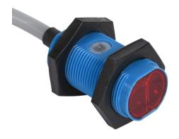
Contrinex photoelectric sensor, tubular, threaded, polarized retroreflective, visible red, 0.02-7m sensing distance, complementary light-on/dark-on, PNP, 4-wire, pigtail.
