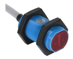
Contrinex photoelectric sensor, tubular, threaded, polarized retroreflective, visible red, 0.02-7m sensing distance, complementary light-on/dark-on, NPN, 4-wire, pigtail.
