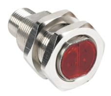
Contrinex photoelectric sensor, tubular, threaded, retroreflective, visible red, 0.02-7m sensing distance, complementary light-on/dark-on, PNP, 4-wire, 4-pin M12 quick-disconnect.
