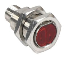
Contrinex photoelectric sensor, tubular, threaded, retroreflective, visible red light emission, 0.02-7m sensing distance, complementary light-on/dark-on, NPN, 4-wire, 4-pin M12 quick-disconnect.
