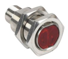
Contrinex photoelectric sensor, tubular, threaded, retroreflective, visible red, 0.02-7m sensing distance, complementary light-on/dark-on, NPN, 4-wire, 4-pin M12 quick-disconnect.
