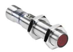
Contrinex photoelectric sensor, tubular, threaded, retroreflective, visible red light emission, 0.15-4m sensing distance, complementary light-on/dark-on, PNP, 4-wire, 4-pin M12 quick-disconnect.
