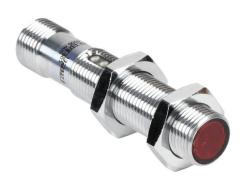
Contrinex photoelectric sensor, tubular, threaded, retroreflective, visible red, 0.15-4m sensing distance, complementary light-on/dark-on, PNP, 4-wire, 4-pin M12 quick-disconnect.
