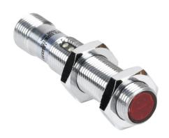
Contrinex photoelectric sensor, tubular, threaded, retroreflective, visible red light emission, 0.15-4m sensing distance, complementary light-on/dark-on, NPN, 4-wire, 4-pin M12 quick-disconnect.
