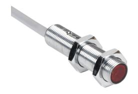
Contrinex photoelectric sensor, tubular, threaded, retroreflective, visible red, 0.15-4m sensing distance, complementary light-on/dark-on, PNP, 4-wire, pigtail.
