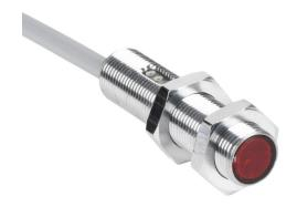
Contrinex photoelectric sensor, tubular, threaded, retroreflective, visible red light emission, 0.15-4m sensing distance, complementary light-on/dark-on, NPN, 4-wire, pigtail.
