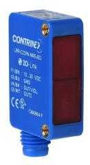
Contrinex photoelectric sensor, rectangular, polarized retroreflective, visible red light emission, 30-6000mm sensing distance, complementary light-on/dark-on, PNP, IO-Link only, 4-wire, 4-pin M8 quick-disconnect.
