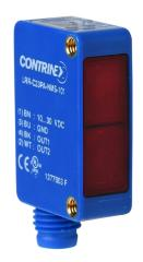
Contrinex photoelectric sensor, rectangular, polarized retroreflective, visible red, 30-6000mm sensing distance, complementary light-on/dark-on, NPN, 4-wire, 4-pin M8 quick-disconnect.
