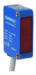
Contrinex photoelectric sensor, rectangular, polarized retroreflective, visible red light emission, 30-6000mm sensing distance, complementary light-on/dark-on, NPN, 4-wire, pigtail.
