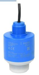
Flowline EchoBeam frequency modulated continuous wave (FMCW) radar liquid and bulk solids level sensor, liquid 32.8ft/10m, solids 16.4ft/5m sensing range, 4-20 mA, 12-30 VDC operating voltage, 1-1/2in male NPT process connection.
