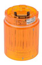
Patlite LED light element, 40mm diameter, yellow, permanent or flashing (60 fpm +/- 2 fpm) light function, 24 VDC, colored lens. For use with LR4 series signal towers.
