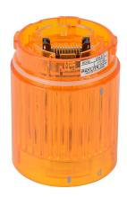
Patlite LED light element, 40mm diameter, yellow, permanent or flashing (60 fpm +/- 2 fpm) light function, 24 VDC, colored lens. For use with LR4 series signal towers.
