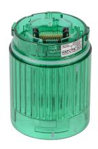
Patlite LED light element, 40mm diameter, green, permanent or flashing (60 fpm +/- 2 fpm) light function, 24 VDC, colored lens. For use with LR4 series signal towers.
