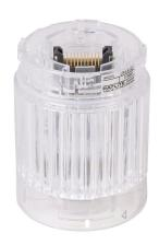
Patlite LED light element, 40mm diameter, green, permanent or flashing (60 fpm +/- 2 fpm) light function, 24 VDC, clear lens. For use with LR4 series signal towers.
