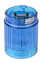
Patlite LED light element, 40mm diameter, blue, permanent or flashing (60 fpm +/- 2 fpm) light function, 24 VDC, colored lens. For use with LR4 series signal towers.
