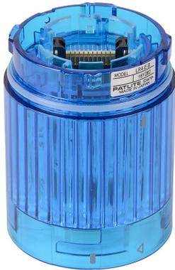
Patlite LED light element, 40mm diameter, blue, permanent or flashing (60 fpm +/- 2 fpm) light function, 24 VDC, colored lens. For use with LR4 series signal towers.
