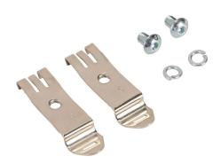
AutomationDirect LR2 series DIN rail adapter, for use with LR2-20P2-1PH, LR2-20P2, LR-20P5, LR2-40xx to LR2-43xx, and LR2-51xx to LR2-52xx line reactors. Clips and mounting hardware included. Allows specified LR2 reactors to be mounted on 35mm DIN rail.
