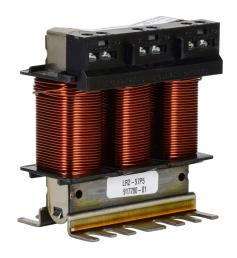
AutomationDirect LR2 series line reactor, 600 VAC, 7-1/2hp, 3-phase, 9A, 3% impedance, input or output side. For use with multiple AC drives.
