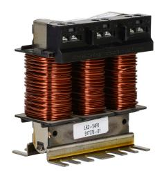
AutomationDirect LR2 series line reactor, 600 VAC, 4hp, 3-phase, 4.9A, 3% impedance, input or output side. For use with multiple AC drives.
