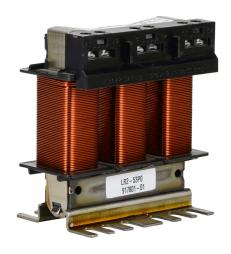
AutomationDirect LR2 series line reactor, 600 VAC, 3hp, 3-phase, 3.9A, 3% impedance, input or output side. For use with multiple AC drives.
