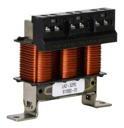
AutomationDirect LR2 series line reactor, 600 VAC, 2hp, 3-phase, 2.7A, 3% impedance, input or output side. For use with multiple AC drives.
