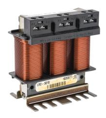
AutomationDirect LR2 series line reactor, 600 VAC, 10hp, 3-phase, 11A, 3% impedance, input or output side. For use with multiple AC drives.
