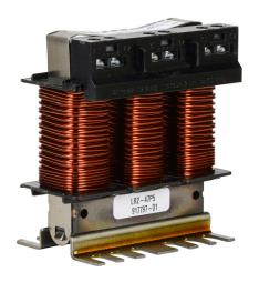
AutomationDirect LR2 series line reactor, 460 VAC, 7-1/2hp, 3-phase, 11A, 3% impedance, input or output side. For use with multiple AC drives.
