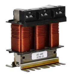
AutomationDirect LR2 series line reactor, 460 VAC, 4hp, 3-phase, 6.2A, 3% impedance, input or output side. For use with multiple AC drives.
