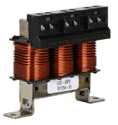
AutomationDirect LR2 series line reactor, 460 VAC, 3hp, 3-phase, 4.8A, 3% impedance, input or output side. For use with multiple AC drives.
