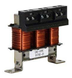
AutomationDirect LR2 series line reactor, 460 VAC, 1-1/2hp, 3-phase, 3A, 3% impedance, input or output side. For use with multiple AC drives.
