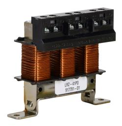
AutomationDirect LR2 series line reactor, 460 VAC, 1hp, 3-phase, 2.1A, 3% impedance, input or output side. For use with multiple AC drives.
