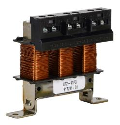
AutomationDirect LR2 series line reactor, 480 VAC, 1hp, 3-phase, 2.1A, 3% impedance, input or output side. For use with multiple AC drives.
