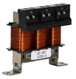
AutomationDirect LR2 series line reactor, 460 VAC, 3/4hp, 3-phase, 1.6A, 3% impedance, input or output side. For use with multiple AC drives.
