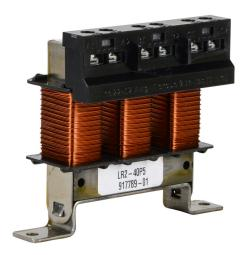
AutomationDirect LR2 series line reactor, 460 VAC, 1/2hp, 3-phase, 1.1A, 3% impedance, input or output side. For use with multiple AC drives.
