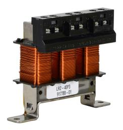
AutomationDirect LR2 series line reactor, 460 VAC, 1/3hp, 3-phase, 0.8A, 3% impedance, input or output side. For use with multiple AC drives.
