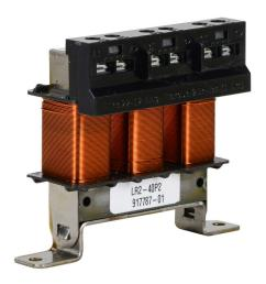
AutomationDirect LR2 series line reactor, 460 VAC, 1/4hp, 3-phase, 0.7A, 3% impedance, input or output side. For use with multiple AC drives.
