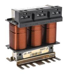
AutomationDirect LR2 series line reactor, 460 VAC, 10hp, 3-phase, 14A, 3% impedance, input or output side. For use with multiple AC drives.
