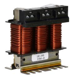
AutomationDirect LR2 series line reactor, 230 VAC, 1-1/2hp, 3-phase, 11A, 3% impedance, input or output side. For use with multiple AC drives.
