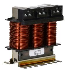
AutomationDirect LR2 series line reactor, 230 VAC, 1hp, 3-phase, 11A, 3% impedance, input or output side. For use with multiple AC drives.
