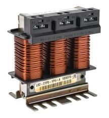
AutomationDirect LR2 series line reactor, 230 VAC, 1hp, 1-phase, 11.6A, 3% impedance, input side only. For use with multiple AC drives.
