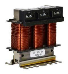
AutomationDirect LR2 series line reactor, 208/240 VAC, 1/2hp, 1-phase, 6.2A, 3% impedance, input side only. For use with multiple AC drives.
