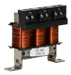
AutomationDirect LR2 series line reactor, 208/240 VAC, 1/4hp, 3-phase, 3A, 3% impedance, input or output side. For use with multiple AC drives.
