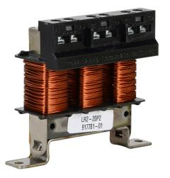
AutomationDirect LR2 series line reactor, 230 VAC, 1/4hp, 3-phase, 3A, 3% impedance, input or output side. For use with multiple AC drives.
