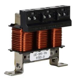
AutomationDirect LR2 series line reactor, 230 VAC, 1/4hp, 1-phase, 3.4A, 3% impedance, input side only. For use with multiple AC drives.
