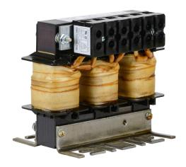
AutomationDirect LR2 series line reactor, 110 VAC, 1hp, 1-phase, 16.7A, 5% impedance, input side only. For use with multiple AC drives.
