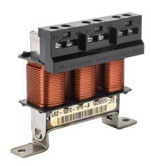
AutomationDirect LR2 series line reactor, 110 VAC, 1/4hp, 1-phase, 10A, 3% impedance, input side only. For use with multiple AC drives.
