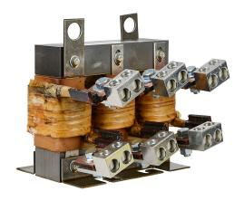
AutomationDirect LR series line reactor, 460 VAC, 250hp, 3-phase, 302A, 3% impedance, input or output side. For use with multiple AC drives.
