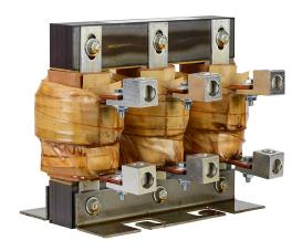
AutomationDirect LR series line reactor, 460 VAC, 150hp, 3-phase, 180A, 3% impedance, input or output side. For use with multiple AC drives.
