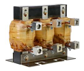
AutomationDirect LR series line reactor, 460 VAC, 100hp, 3-phase, 124A, 3% impedance, input or output side. For use with multiple AC drives.
