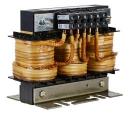
AutomationDirect LR series line reactor, 460 VAC, 60hp, 3-phase, 77A, 3% impedance, input or output side. For use with multiple AC drives.
