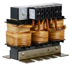
AutomationDirect LR series line reactor, 460 VAC, 40hp, 3-phase, 52A, 3% impedance, input or output side. For use with multiple AC drives.
