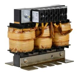
AutomationDirect LR series line reactor, 460 VAC, 30hp, 3-phase, 40A, 3% impedance, input or output side. For use with multiple AC drives.
