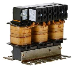
AutomationDirect LR series line reactor, 460 VAC, 20hp, 3-phase, 27A, 3% impedance, input or output side. For use with multiple AC drives.
