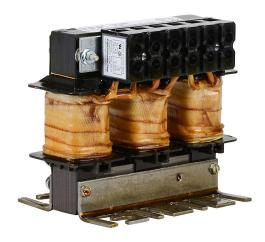
AutomationDirect LR series line reactor, 230 VAC, 7-1/2hp, 3-phase, 24.2A, 3% impedance, input or output side. For use with multiple AC drives.
