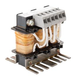
AutomationDirect LR series line reactor, 230 VAC, 3hp, 3-phase, 10.6A, 3% impedance, input or output side. For use with multiple AC drives.
